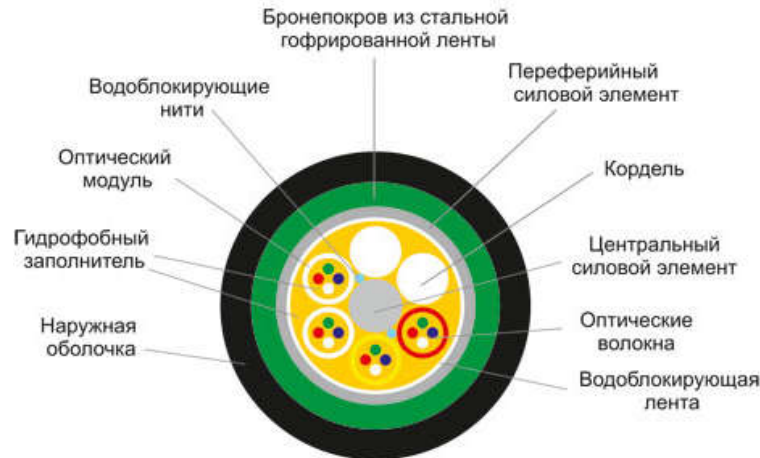
Figure 12. An example of FOC construction for installation in buildings
